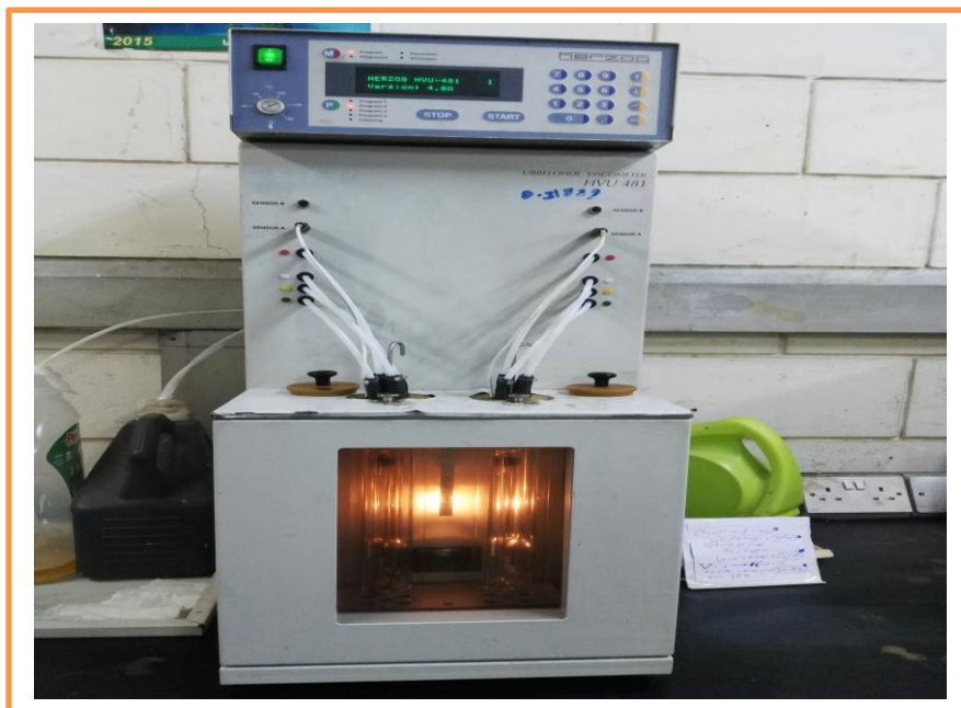
Figure ( 2.1) : Device of the kinematic viscosity measurement
