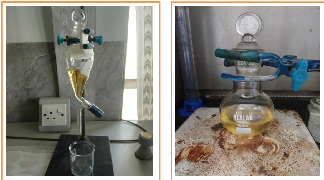
Figure ( 2.9 ) : The oil after distillation with solvents
