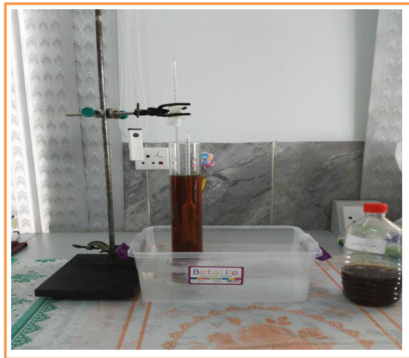
Figure (2.2) : Hydrometer for specific gravity measurements
