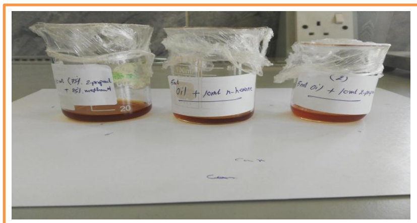
Figure ( 2.8 ) : The oil after distillation with solvents
