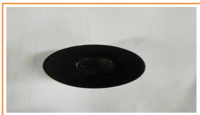
Figure (2.6) : The carbon residue after being heated by Bunsen burner
