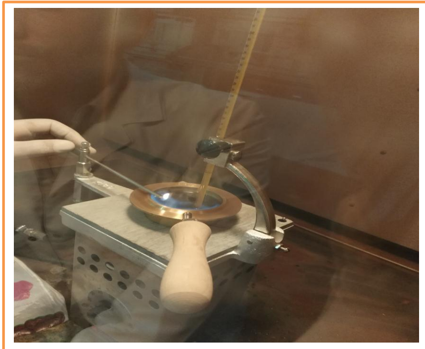
Figure (2.3 ) : Device of the flash point measurement
